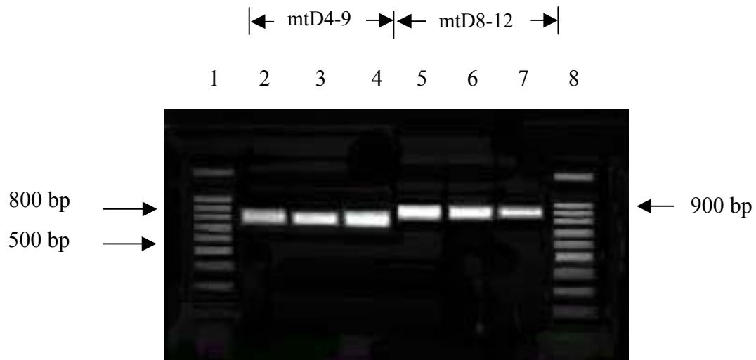
Figure 21. The PCR product of about 800 bp of COI gene amplified by using primers mtD-4 and mtD-9 (lane 2-4), and primers mtD-8 and mtD-12 (lane 5-7). The 100-bp markers are shown in lanes 1 and 8.
