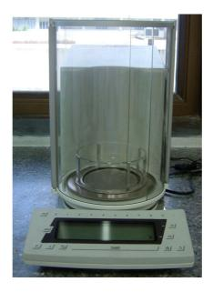
Fig.24: Digital scale analytical balance (Sortarius model MC 210S)
