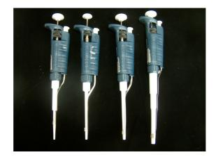
Fig.23: Precision pipettors 20, 100, 200 and 1,000  $\mu l$
