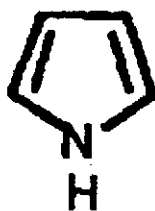
Fig. 4.2. The chemical structure of conducting monomer used to prepare polypyrrole film
