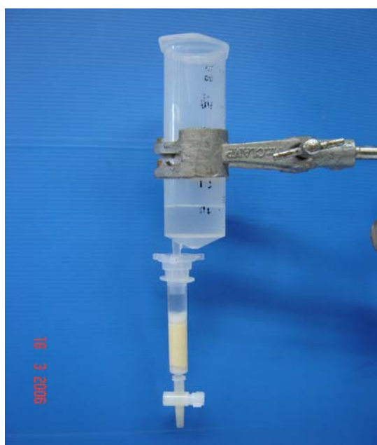
Figure 2-1 Preparation of Amberlite IRC-748 resin column
