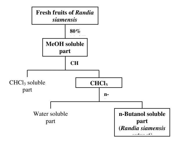
Figure 16 Flow chart showing preparation of n-butanol extract from fresh fruits of *Randia* siamensis
