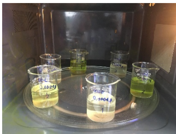
Figure 4 Extraction of R. nasutus using microwave extraction technique
