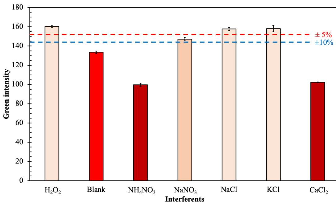
**Figure 26** The green intensity of colorimetric product produced from hydrogen peroxide detection in the presence of various interferences, under optimized condition. The concentrations of hydrogen peroxide and interferences in the respective mixture were 300 mmol L<sup>-1</sup>. (n=3)
