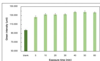
Figure 3 Green intensity values of APTES-GA probes after immersion in 1 mL of 200 mM hydrogen peroxide solution for 5, 10, 20, 30, 40, 50 and 60 minutes.
