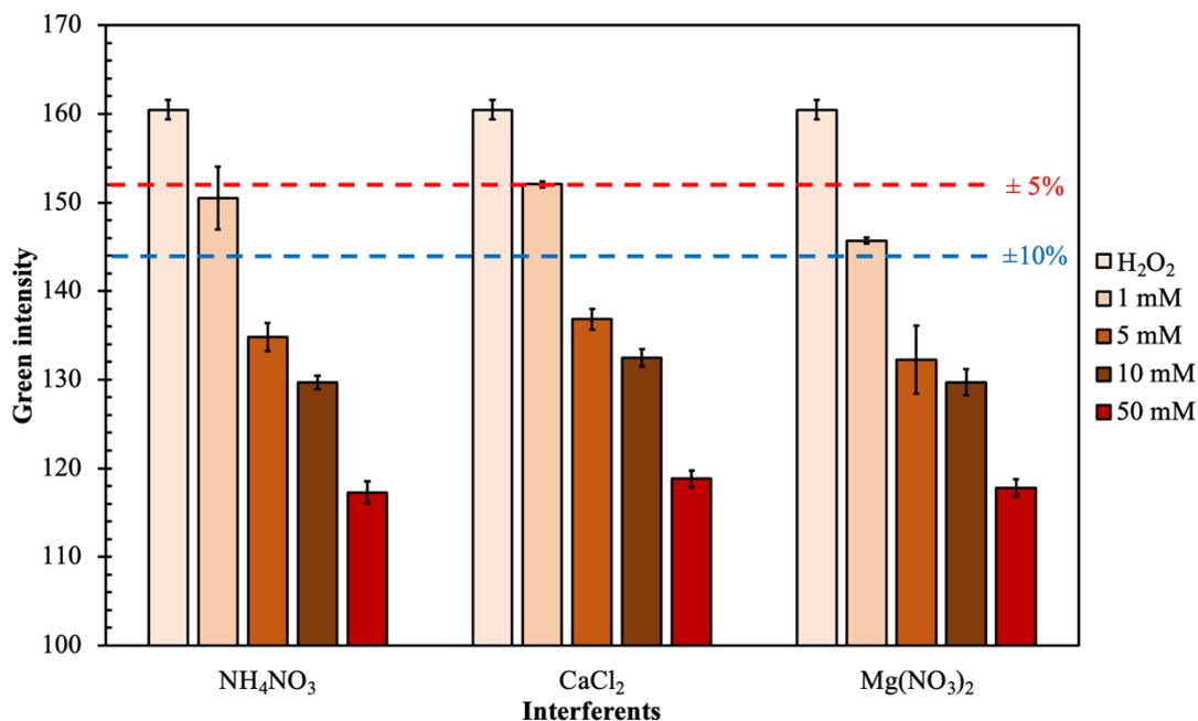
**Figure 27** The green intensity of resulting probe obtained from hydrogen peroxide detection in various concentrations of interferences. (n=3)
