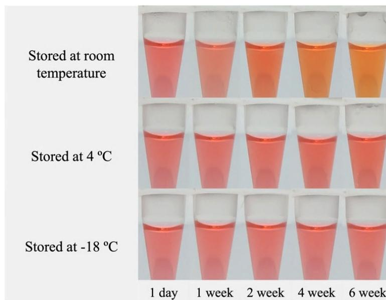
**Figure 28** The APTES-GA probe after stored at three different conditions: room temperature, 4 °C, and -18 °C.
