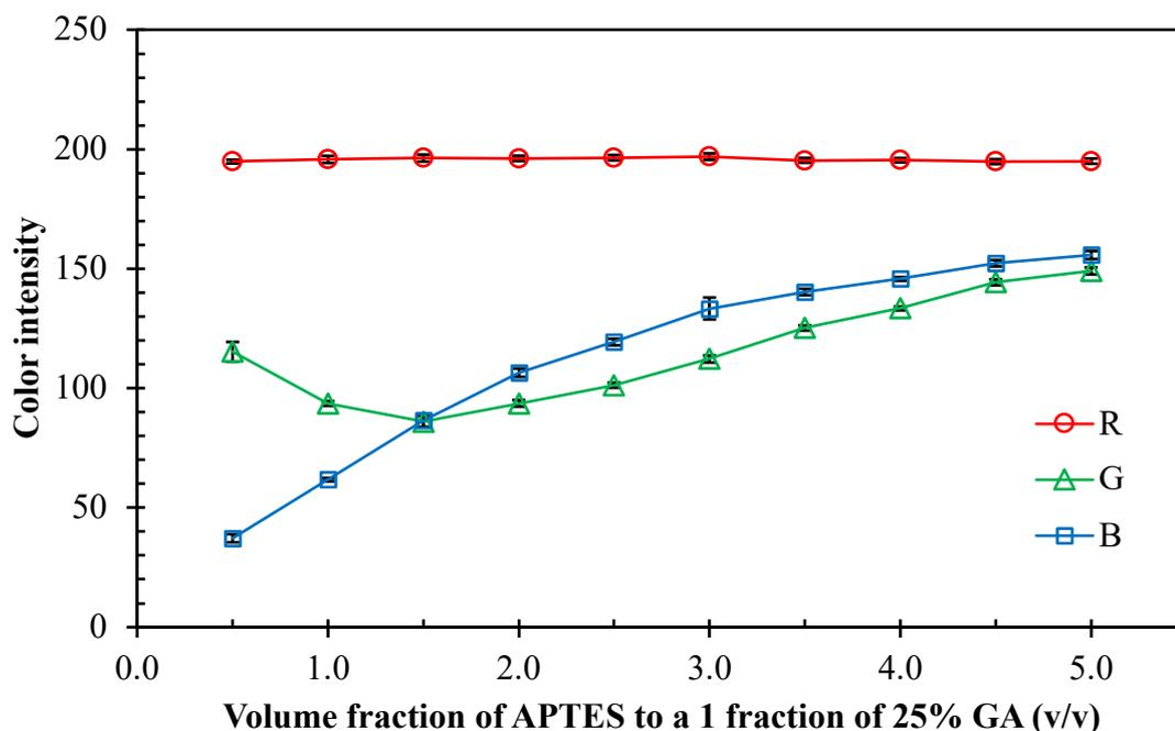
**Figure 6** The plot of color intensity against the volume fraction of APTES per 1 fraction of 25% GA solution. The APTES-GA solution was incubated for 24 hours before measurement. (n=3)
