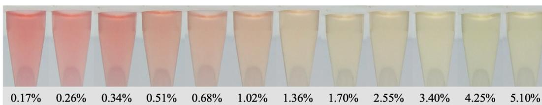
**Figure 21** The pictures of APTES-GA probe after a treatment by hydrogen peroxide solution varying from 0.003 %w/v to 5.10 %w/v.
