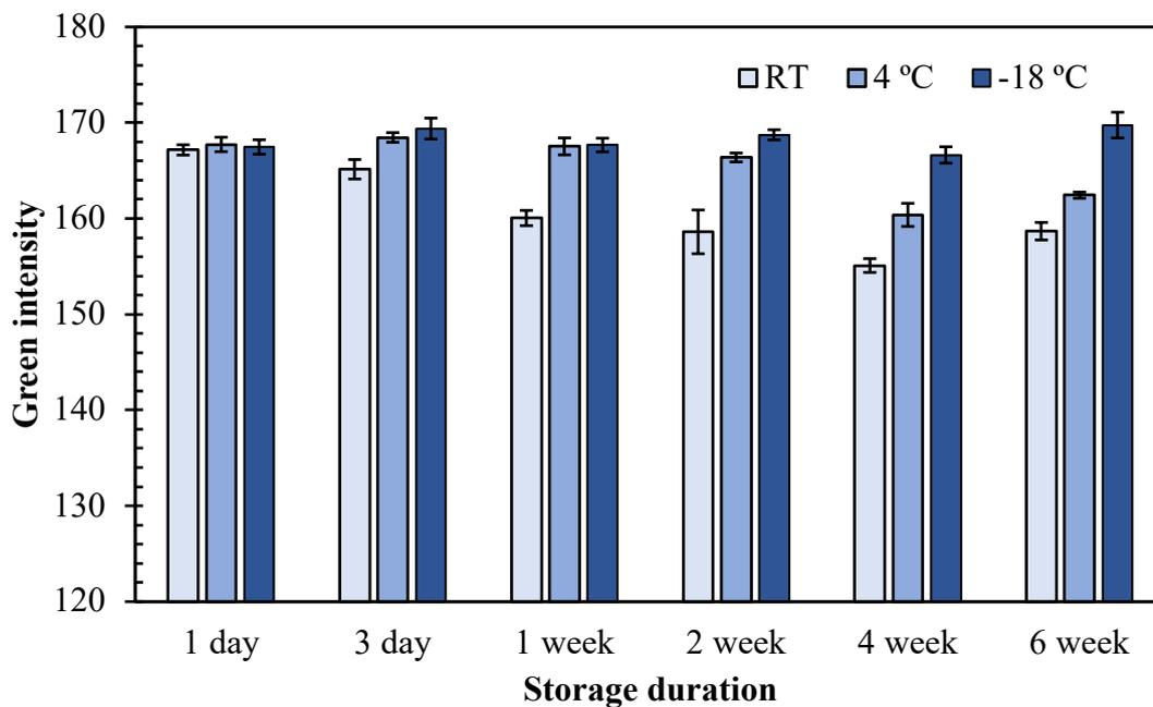
**Figure 29** The green intensity of colorimetric products obtained from APTES-GA probes stored at three different conditions: room temperature, 4 °C, and -18 °C. (n=3)
