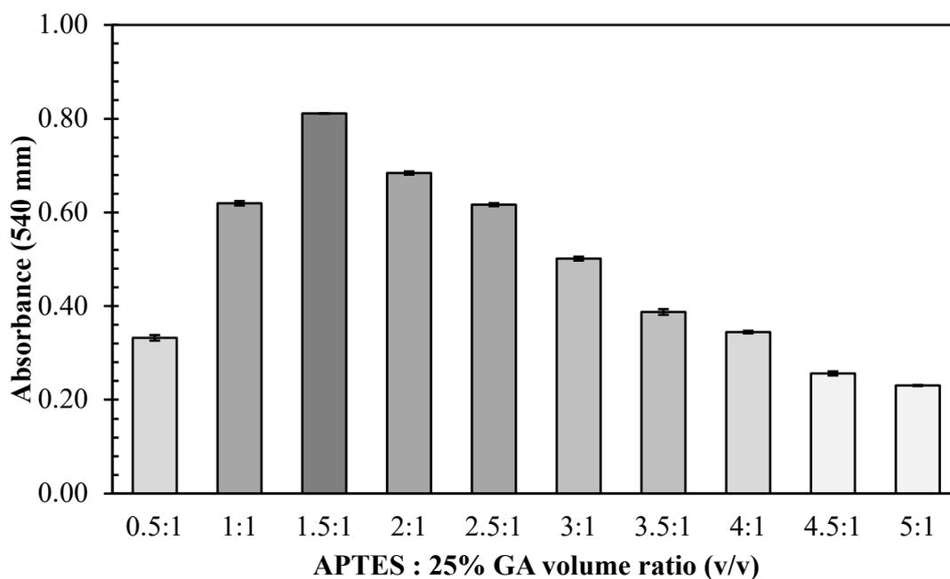
**Figure 8** The absorbance at 540 nm of each APTES : 25% GA volume ratio. (n=3)
