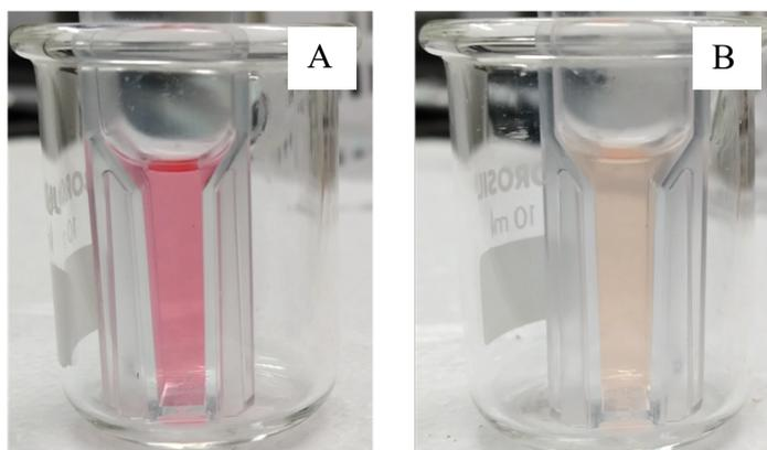
**Figure 12** (A) The pictures of APTES-GA complex solution treated ethanol blank at a volume ratio of 3:7 v/v. (B) The picture of APTES-GA complex solution treated with  $300 \text{ mmol L}^{-1}$  (1.02 %w/v) hydrogen peroxide solution at a volume ratio of 3:7 v/v and the reaction time was 5 minutes.
