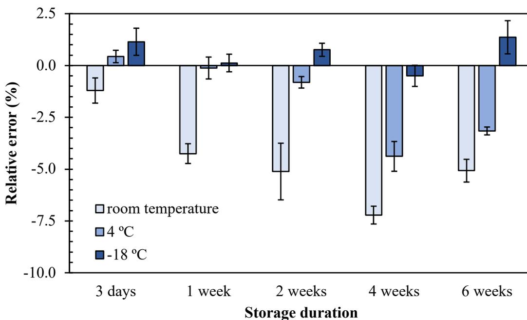
**Figure 30** The relative error of green intensity of colorimetric products from APTES-GA probes stored at three different conditions: room temperature, 4 °C, and -18 °C. (n=3)
