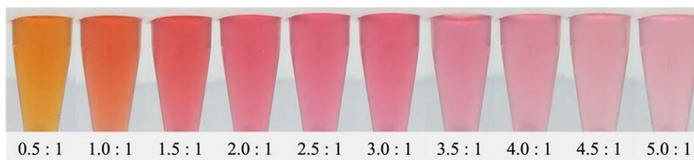
**Figure 5** Digital images of APTES-GA probes that were prepared from APTES and 25% GA solution at volume ratio ranged from 0.5:1 to 5.0:1 v/v. The image was captured after the incubation time of 24 hours.
