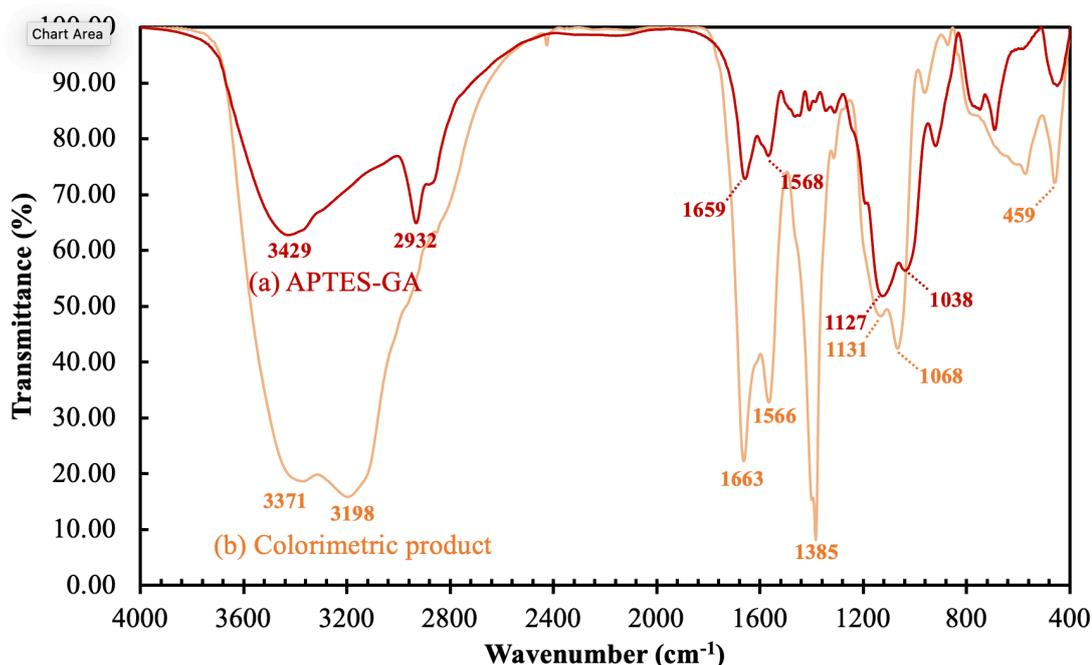
**Figure 14** The FT-IR spectra of solid (a) APTES-GA complex and solid (b) colorimetric product.
