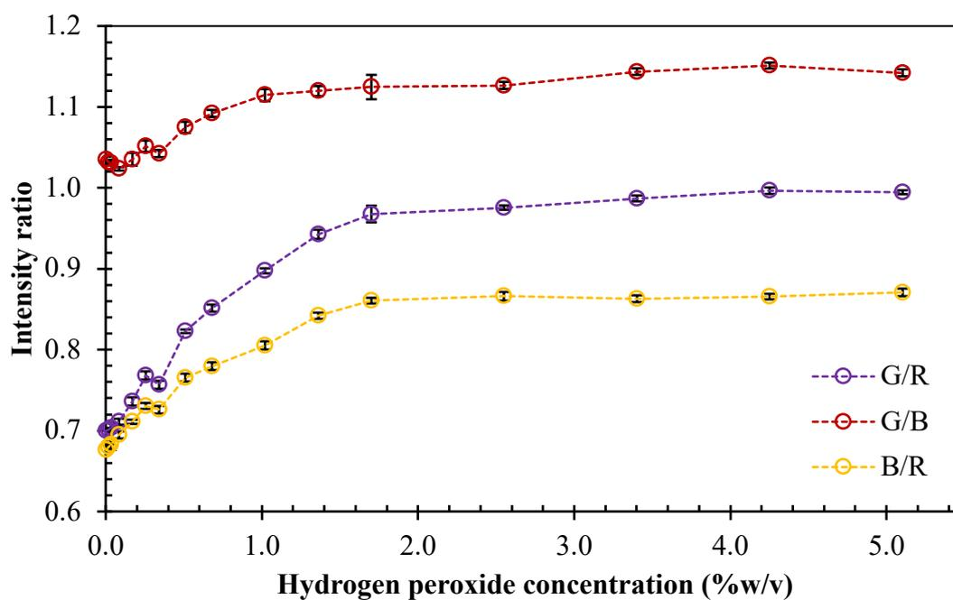
**Figure 24** The plot of intensity ratio of resulting probe against hydrogen peroxide concentrations in a range of 0.003 %w/v - 5.10% w/v. (n=7)
