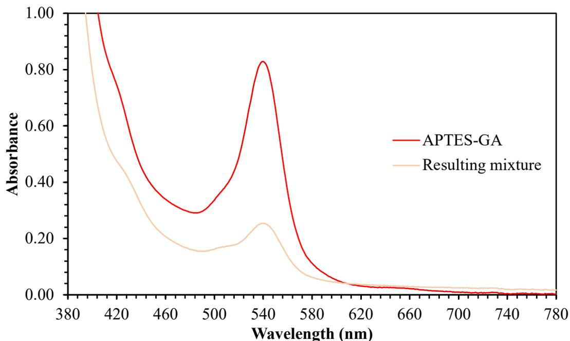
**Figure 13** The UV-visible absorption spectra of APTES-GA solution after treatments with reagent blank (acetonitrile) and 300 mmol L<sup>-1</sup> (1.02 %w/v) hydrogen peroxide solution for 5 minutes. The volume ratio of APTES-GA to treating solution was 3:7 v/v.
