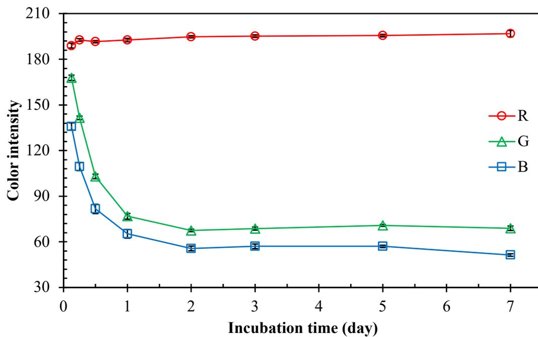
**Figure 10** The plot of color intensity of APTES-GA probe against incubation time. (n=3)
