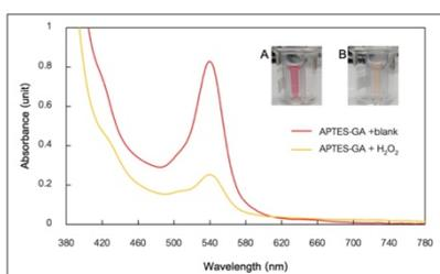
**Figure 1** UV-Visible absorption spectra of reagent blank (700  $\mu$ L) with APTES-GA complex solution (300  $\mu$ L) (red line) and the oxidation reaction of 300 mM hydrogen peroxide solution (700  $\mu$ L) with APTES-GA complex solution (300  $\mu$ L) (yellow line). The spectra were measured at 5 min after mixing.
