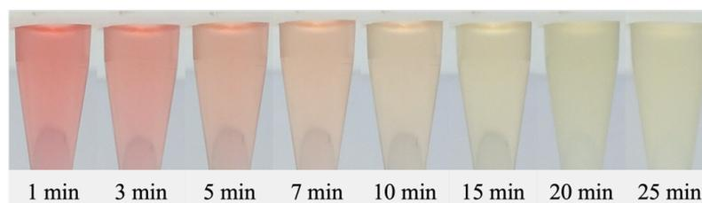
**Figure 19** The pictures of APTES-GA probes after a treatment with  $750 \text{ mmol L}^{-1}$  ( $2.55 \text{ \%w/v}$ ) hydrogen peroxide solution. The volume ratio of APTES-GA : analyte solution was 1:1 v/v and the observation time started from 1 minute to 25 minutes. ( $n=3$ )
