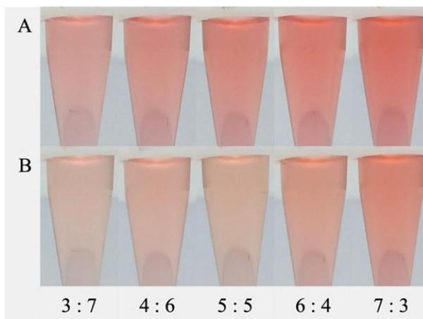
**Figure 16** The APTES-GA probes after treatment with (A) blank (acetonitrile) and (B)  $750 \text{ mmol L}^{-1}$  (2.55 %w/v) hydrogen peroxide solution. The volume ratio of APTES-GA : hydrogen peroxide solution was ranged from 3:7 to 7:3 v/v (left to right). The reaction time was 7 minutes. (n=3)
