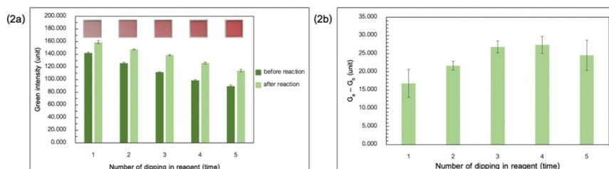
Figure 2 (2a) Green intensity values of APTES-GA probes which adsorbed APTES-GA complex at different amounts (dark green column) and green intensity values of APTES-GA probes after immersion in 1 mL of 200 mM hydrogen peroxide solution (pale green column). (2b) The differences of green intensity values of APTES-GA probes before ( $G_b$ ) and after reaction ( $G_a$ ). Note: The difference between the green values of the APTES-GA probes before and after reaction was  $G_a - G_b$ .
