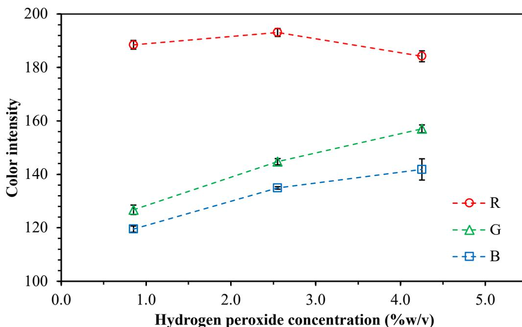
**Figure 15** The plot of color intensity of APTES-GA probe after treatment with hydrogen peroxide solution. The volume ratio of APTES-GA : analyte solution was 1:1 v/v, and the reaction was 7 minutes. (n=3)
