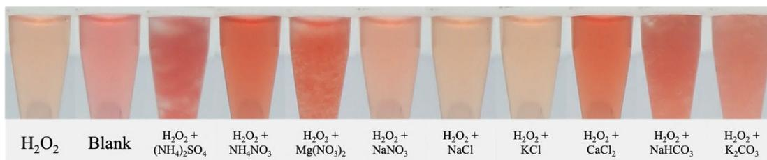
**Figure 25** The colorimetric product obtained from APTES-GA probe that was treated with hydrogen peroxide detection in the presence of various interferences. The concentration of hydrogen peroxide and interferences in the respective mixture were 300 mmol L<sup>-1</sup>.
