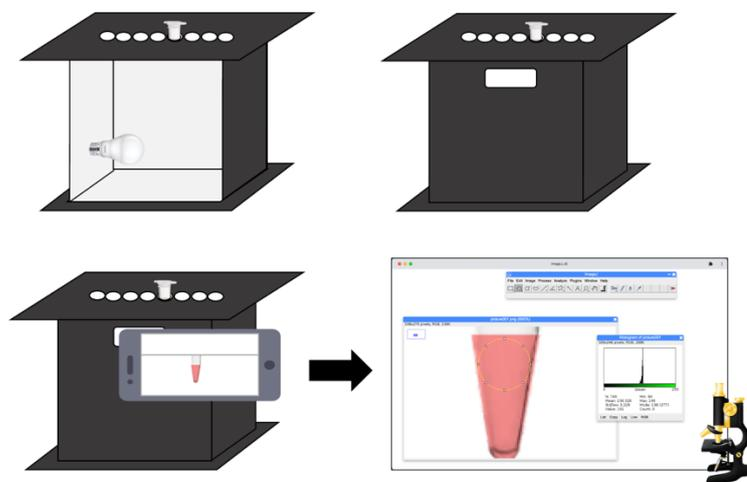
**Figure 3** The picture illustrated the custom-build photographic box and digital image processing with a smartphone as an image capturing device.
