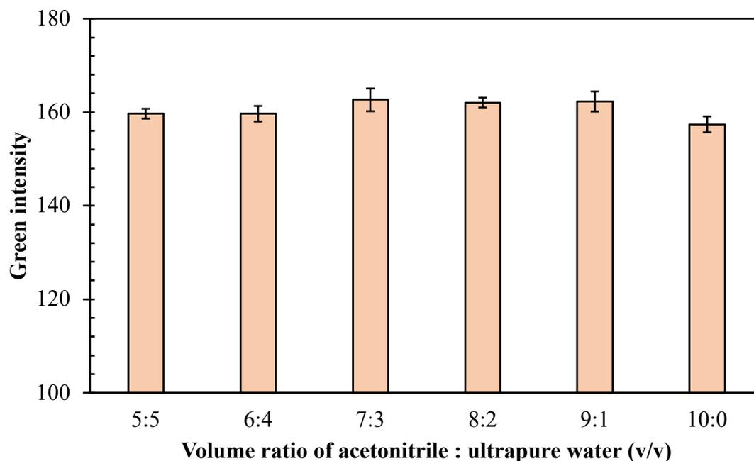
**Figure 18** The green intensity of colorimetric product obtained by a treatment of 750 mmol L<sup>-1</sup> (2.55 %w/v) hydrogen peroxide solution in medias that has acetonitrile : water ranged from 5:5 to 10:0 v/v. The volume ratio of APTES-GA : analyte solution was 1:1 v/v, and the reaction time was 7 minutes. (n=3)
