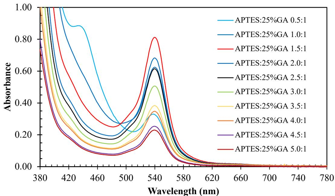
**Figure 7** The absorption spectra of five-fold diluted APTES-GA complex solutions that were prepared with APTES : 25% GA volume ratios varying from 0.5:1 to 5.0:1 v/v.
