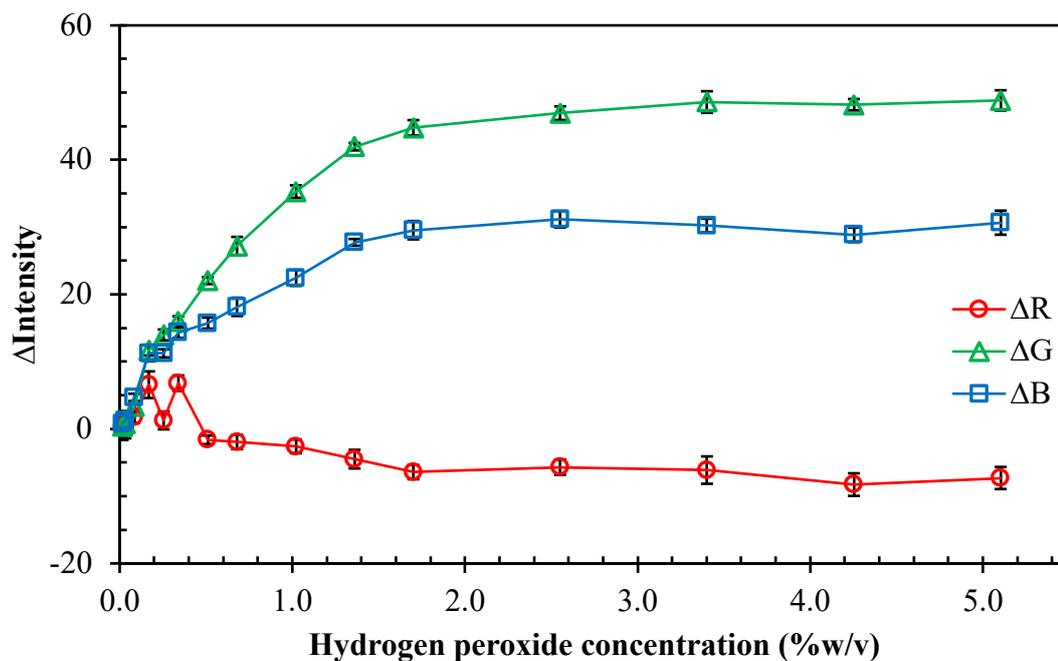
**Figure 23** The plot of difference of color intensity ( $\Delta$ intensity) of resulting probe and blank against hydrogen peroxide concentrations in a range of 0.003 %w/v - 5.10% w/v. (n=7)
