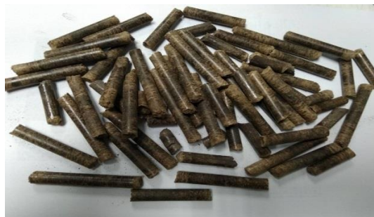
Figure 3. 2 Fuel Pellet (50%sewage sludge + 50%wood sawdust).
