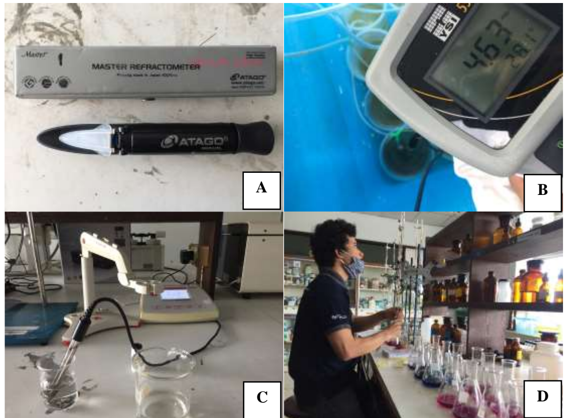
Figure 2.4 The measurements of dissolved oxygen, temperature and pH.
