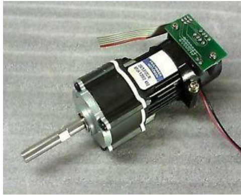
(a) Faulhaber 12V-DC motor with encoder [58]
