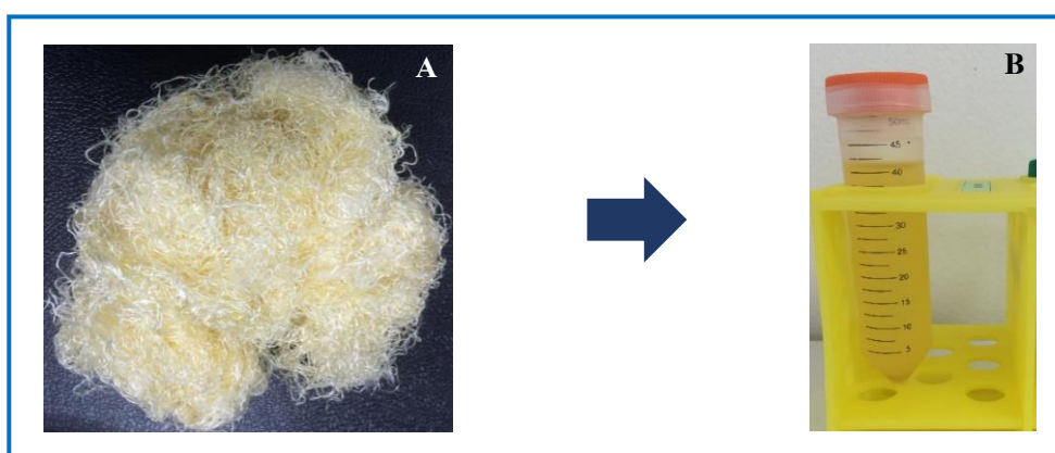
Figure 7. Picture of degummed silk fibroin (A) and silk fibroin aqueous solution (B)
