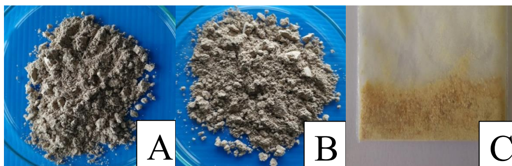
Figure 3.1 Hemicellulose from sterilizer condensate (HSC) (A), decanter effluent (HDE) (B) of palm oil mill waste and commercial xylan from beech wood (CXB) (C)
