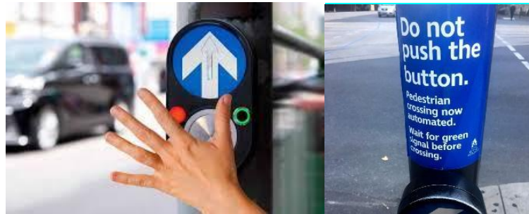
Figure 4.33 The contactless pedestrian crossings, Adelaide 54 (C1)
