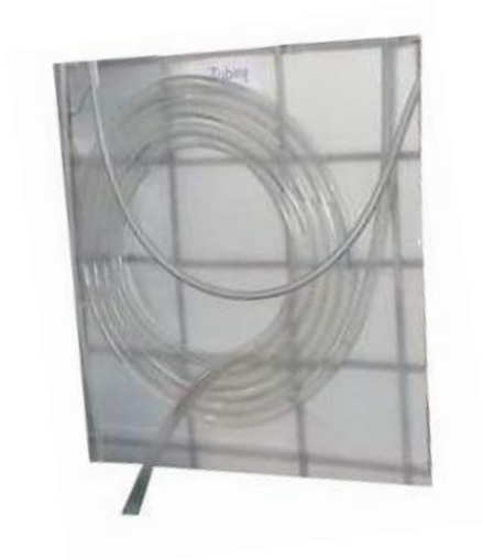
Figure 3.17 Tube absorber for separated CO 2 from biogas.
