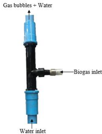
Figure 3.14 Microbubble generator system.
