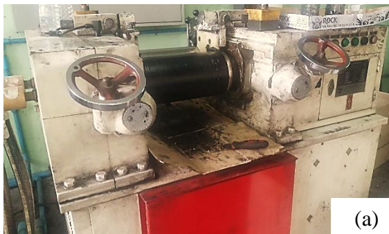
Figure 20 (a) Two-roll mill machine; (b) Hydraulic hot press machine
