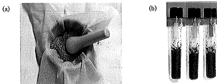
Figure 25. Screening of cyanogenic plant by picrate paper test. (a) Ground plant sample in liquid nitrogen by pestle and mortar. (b) The change in color of picrate paper from yellow to orange/red showed occurrence of HCN liberated from crushed plant materials.
