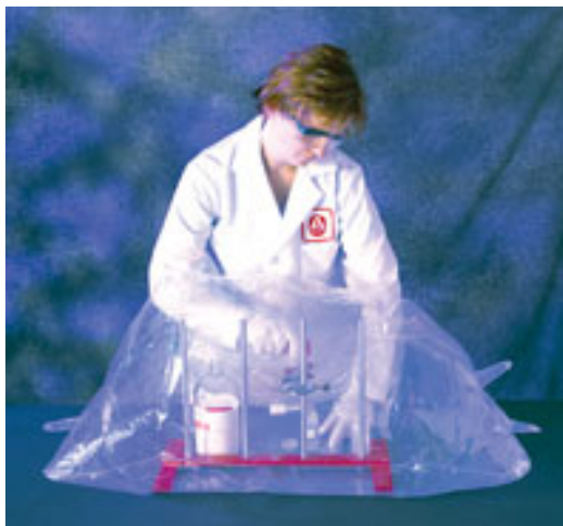
Figure 3-16 Two-hand anaerobic glove bag (Aldrich ® AtmosBag, from www.sigma-aldrich.com )
