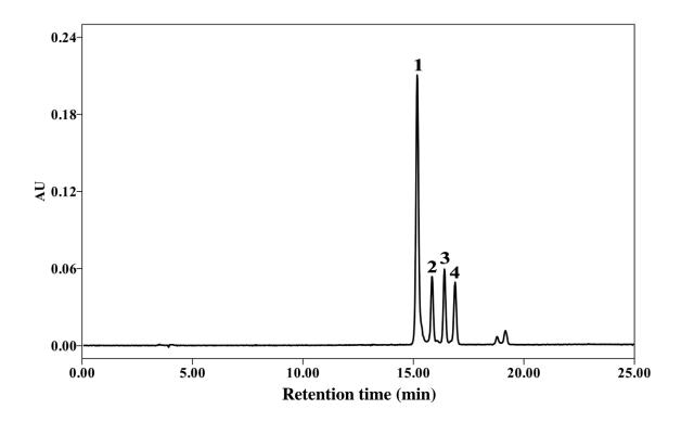
Figure 14. HPLC chromatogram of carotenoids produced by selected strains separated by HPLC using an Inertsil ODS-3  $C_{18}$  reversed-phase column (4.6 mm × 250 mm).
