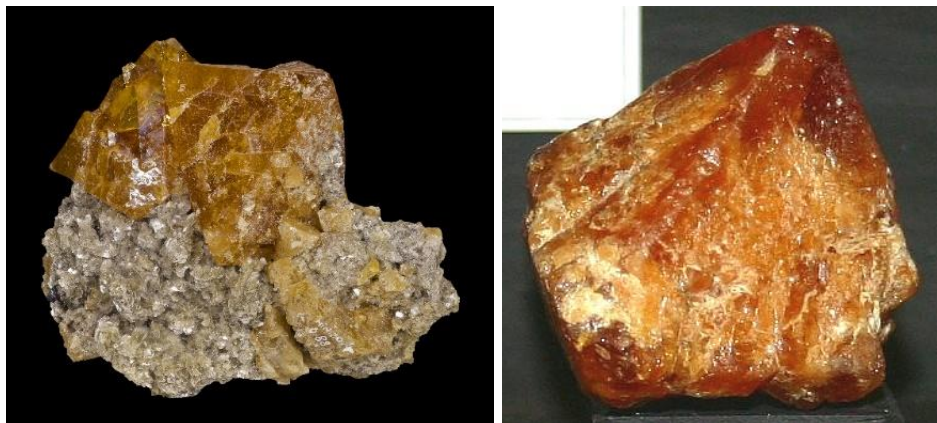
Figure 2.4. Scheelite ( \text{CaWO}_4 ) raw materials [43].
