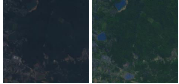
Fig.4 RGB composition of original bands (left) and band ratios of R_{1/2} , R_{2/3} , and R_{2/4} (right).
