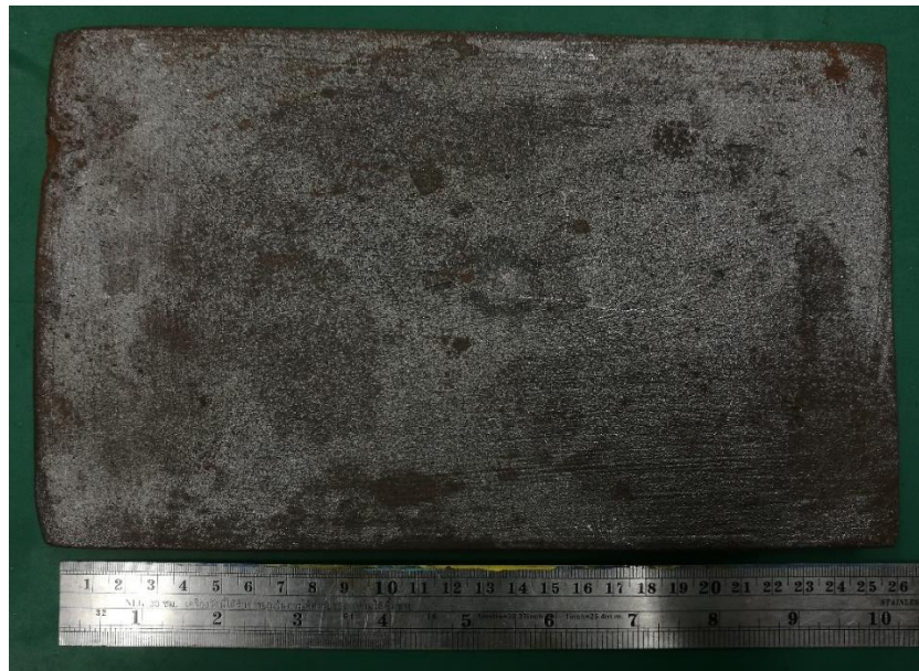
Fig 3.1 3.5% Cr steel plate
