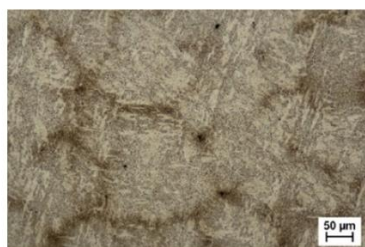
Fig. 2. Microstructure of base metal (3.5% Cr Steel).
