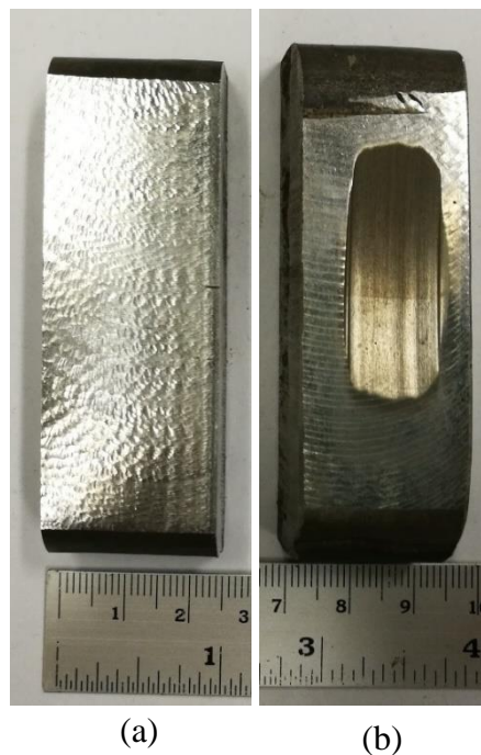
Fig 3.38 The abrasion specimen (a) before testing (b) tested specimen
