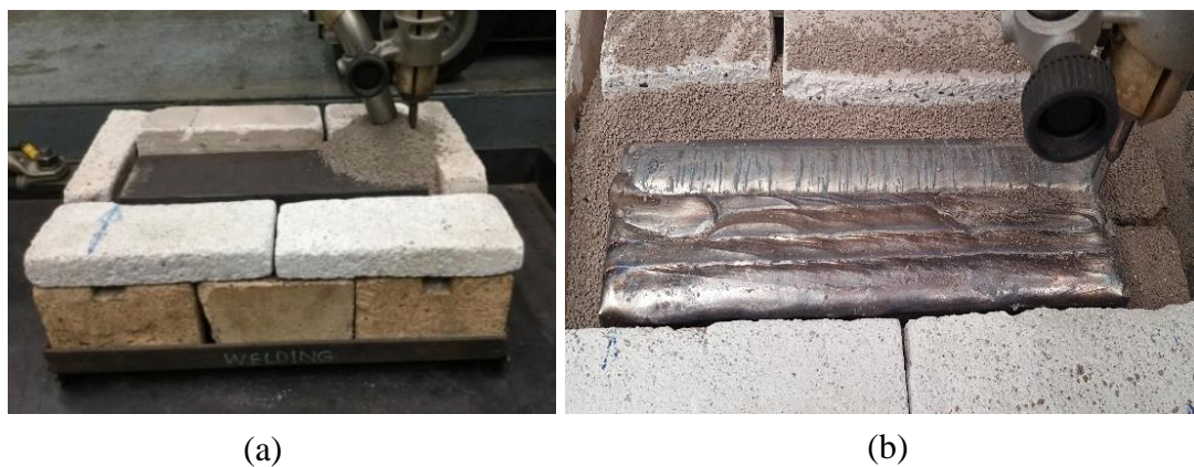
Fig 3.21 Conducting welding process (a) initiating the welding process (b) hardfacing applied to the buffer layer
