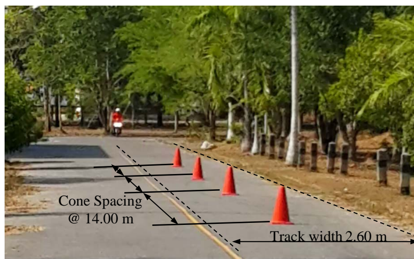
Figure 3.11 Cone Spacing and Track Width
