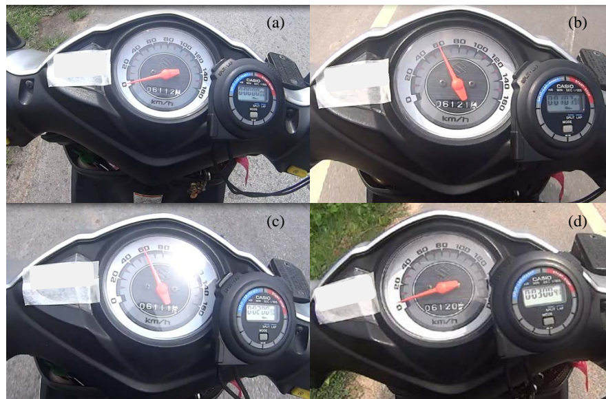
Figure 3.6 Motorcycle Speedometer on Instrument Calibration (a) at starting time 0 sec, (b) at time 60 sec, (c) at time 120 sec, and (d) at time 180 sec
