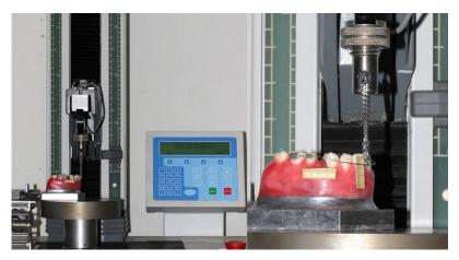
Fig. 14 Universal testing machine and testing method
