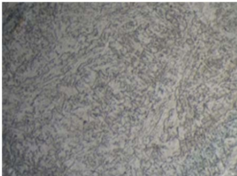
Figure 8 The microstructure at the sprayed surface which was expanded 20 times.
