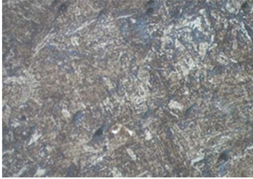
Figure 7 The microstructure at the heat affected zone which was expanded 50 times.
