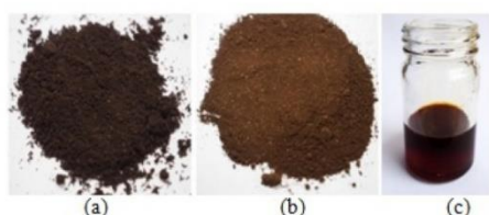
Figure-1. (a) spent coffee grounds, (b) oil-free spent coffee grounds, and (c) coffee oil.
