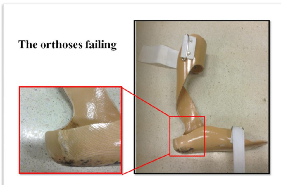
Figure 4.20 The orthoses failing
