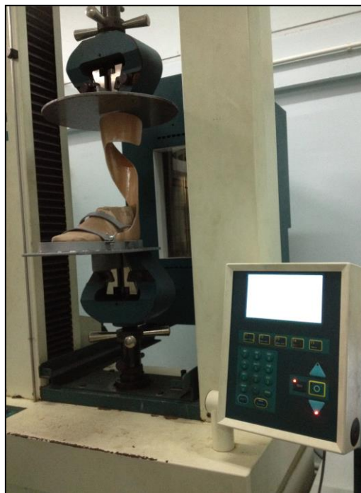
Figure 3.19 Hounsfield Machine (test vertical force of orthoses)
