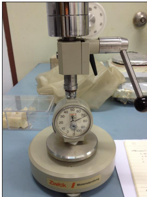
Figure 3.12 The Shore D hardness scales of Zwick Hardness Testing Machine
