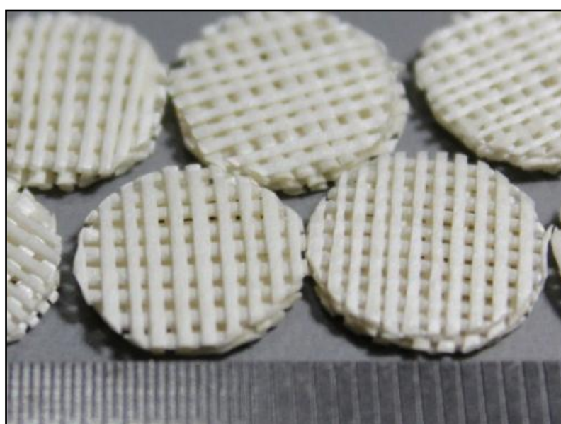
Fig. 1 The picture of the PCL- 20%CS MSMD scaffolds prepared for the experiment.
