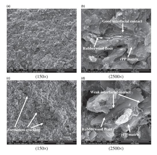
**Figure 6.** SEM micrographs of rPP-rubberwood flour composites showing formation of cracks and interfacial contact between wood flour and plastic matrix (Magnification  $150 \times$  and  $2500 \times$ ): (a), (b) before creep testing and (c), (d) after creep testing.
