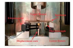
Figure 1. Test apparatus of three-point bending creep.
