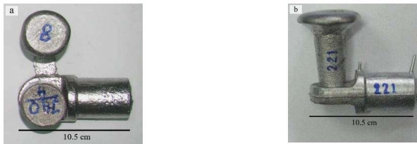
Fig.6 Casting parts prepared by conventional casting (a) and semi-solid casting (b)
