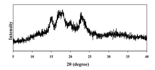
Figure 4. X-ray diffractograms of rice starch powder.
