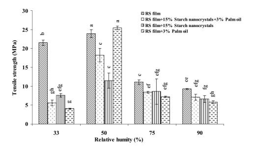
Figure 20. The tensile strength of rice starch film, rice starch film reinforced with starch nanocrystals 15%, rice starch film added with 3% palm oil and rice starch film (RS) reinforced with starch nanocrystals 15% and added with 3% palm oil at various relative humidities (27±2 °C). Mean values with different letter are significantly different (p<0.05).
