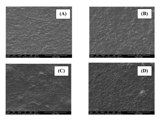
Figure 17. Surface of rice starch film reinforced with starch nanocrystals 15% and added various types of lipid; (A) palm oil 3%, (B) palm oil 6%, (C) palm oil 9% and (D) palm oil 12%.
