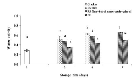
Figure 24 Effect of type of wrapping materials on water activity evaluation with storage time of wrapped cracker condition at 75% RH and room temperature (27±3°C). Mean value with different letter are significant different (p<0.05).
