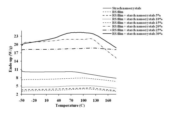
Figure 12. DSC curve of starch nanocrystals, rice starch films (RS) and rice starch films reinforced with starch nanocrystals 5-30%.
