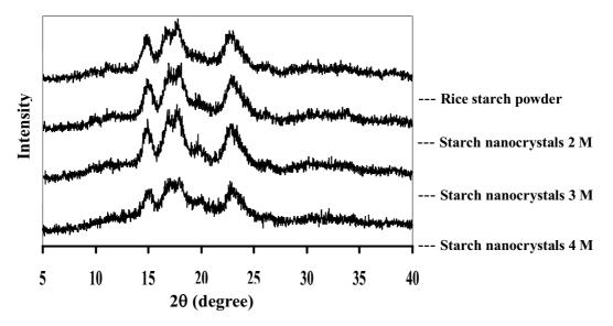
Figure 6. X-ray diffractograms of rice starch powder, starch nanocrystals hydrolysis by sulfuric acid at concentration 2, 3 and 4 M.
