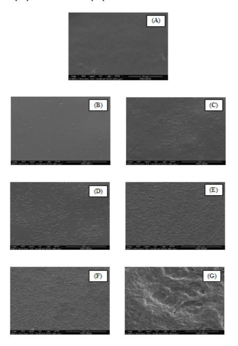
Figure 13. Surface of rice starch films (A), rice starch films reinforced with 5% (B), 10% (C), 15% (D), 20% (E), 25% (F), 30% (G) of starch nanocrystals.
