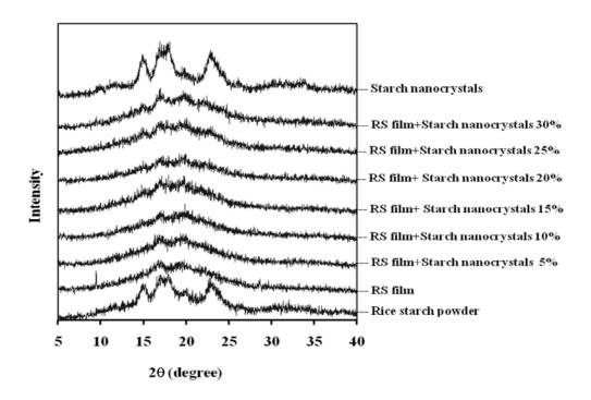
Figure 9. X-ray diffractograms of rice starch powder, starch nanocrystals and rice starch films (RS) reinforced with starch nanocrystals 5-30%.
