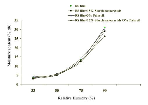
Figure 19. Moisture sorption isotherm curves of rice starch film, rice starch film (RS) reinforced with starch nanocrystals 15%, rice starch film added with 3% palm oil and rice starch film reinforced with starch nanocrystals 15% and added with 3% palm oil at various relative humidities (27±2 °C).
