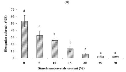
Figure 7.Effect of content of starch nanocrystals on tensile strength (A) and elongation at break (B) of rice starch films. Mean values with different letter are significantly different (p<0.05).
