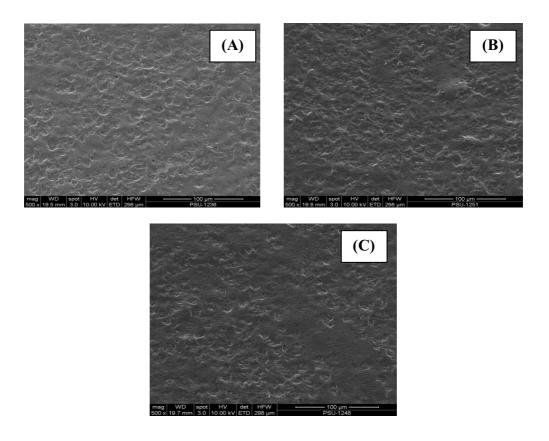
Figure 18. Surface of rice starch film reinforced with starch nanocrystals 15% and added of (A) palm oil 3%, (B) Margarine 3% and (C) Rice bran oil 3%.
