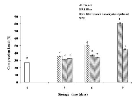
Figure 21 Effect of type of wrapping materials on compression load of wrapped cracker using rice starch film (RS), rice starch film reinforced with starch nanocrystals and added lipid and polyethylene condition at 75% RH and room temperature (27±3°C). Mean value with different letter are significant different (p<0.05).
