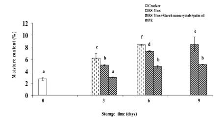
Figure 23 Effect of type of wrapping materials on moisture content evaluation with storage time of wrapped cracker condition at 75% RH and room temperature (27±3°C). Mean value with different letter are significant different (p<0.05).
