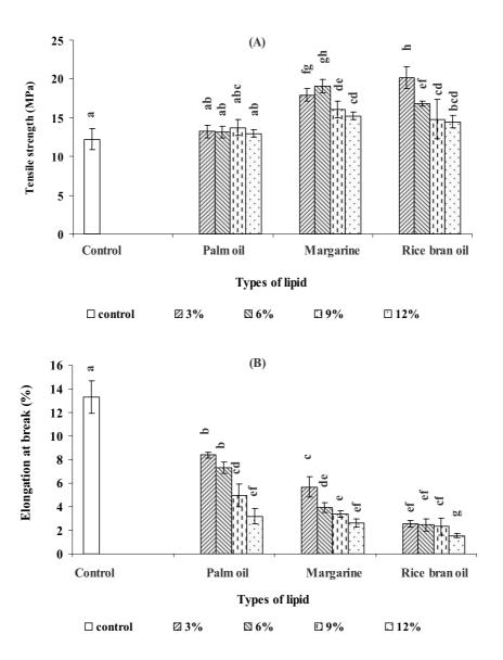
Figure 14. Effect of lipid type and concentration on tensile strength (A) and elongation at break (B) of rice starch films reinforced with starch nanocrystals. Mean values with different letter are significantly different (p<0.05).
