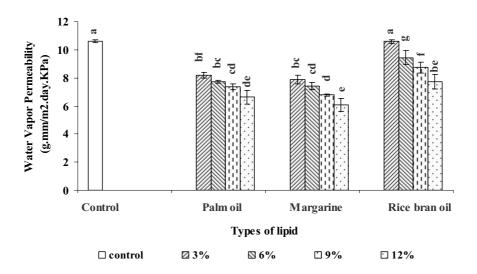
Figure 15. Effect of types and content of lipid on water vapor permeability of rice starch films reinforced with starch nanocrystals. Mean values with different letter are significantly different (p<0.05).
