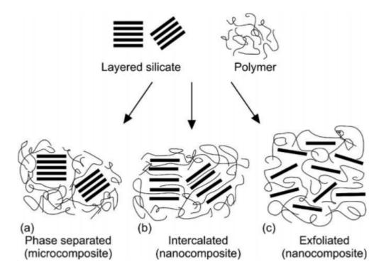
Figure 2. Types of composite derived from interaction between clays and polymer: (a) phase-separated microcomposite; (b) interacalated nanocomposite and (c) exfoliated nanocomposite.
