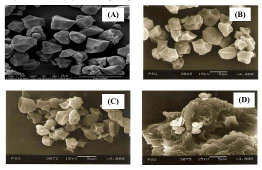
Figure 5. Scanning electron microscope (SEM) of rice starch (A), starch nanocrystals hydrolysis by sulfuric acid at concentration 2 M (B), 3 M (C) and 4 M (D).
