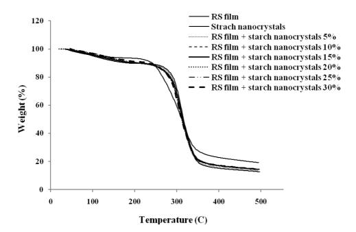
Figure 10. TGA thermograms of starch nanocrystals, rice starch (RS) films and rice starch film reinforced with starch nanocrystals 5-30%.
