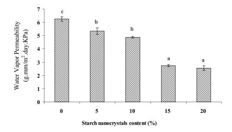
Figure 8. Effect of content of starch nanocrystals on water vapor permeability of rice starch films. Mean values with different letter are significantly different (p<0.05).
