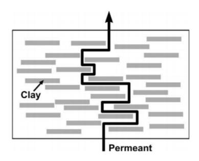
Figure 1. Tortuous path of a permeant in a clay nanocomposite.
