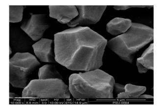
Figure 3. SEM photograph of rice starch granules (scale bar: 5µm).
