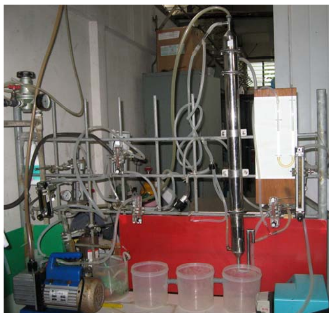
Figure 3.2 Laboratory packed column used for H 2 S removal from gas stream
