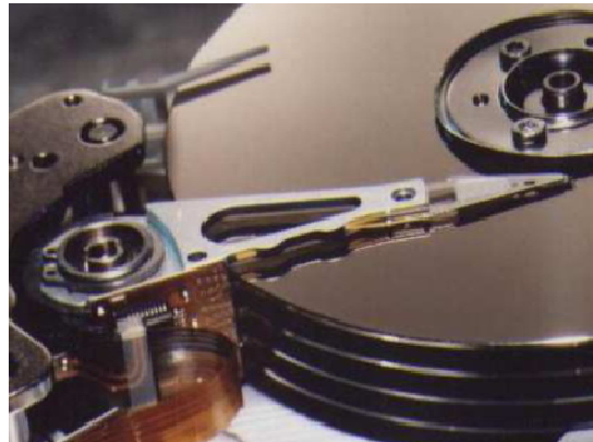
Figure 1-1. Hard disk internals [1].
