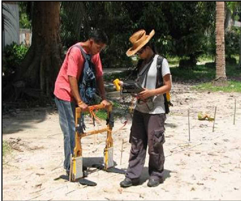
Figure 2.3 GPR measurement at Wat Mo Khlan archaeological site.
