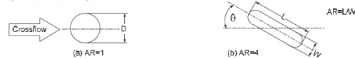
Fig. 2. Orifice geometry with identical area cross-section ( AR is length over width of orifice)
