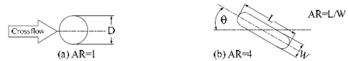
Fig.2 Orifice geometry with identical exit area ( AR is ratio of length over width of orifice)
