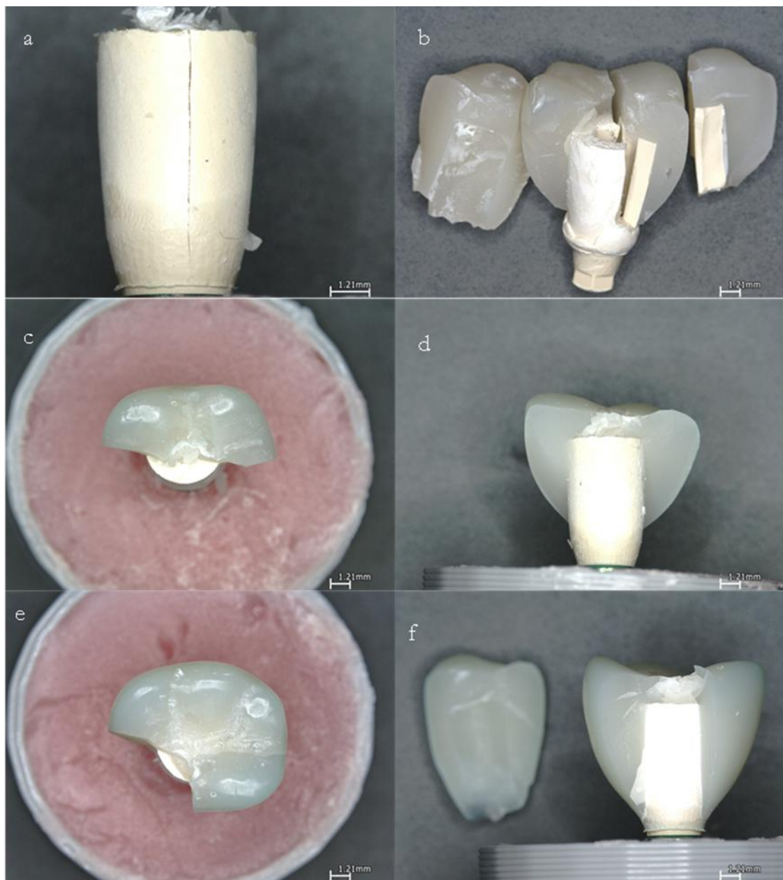
Figure 19 (a) Specimen showing adhesive failure and abutment fracture from the Sa group, and (b) specimen showing cohesive failure from the HA group (c) Specimen showing Type 1 failure from the Sa PEEK group (occlusal view), and (d) specimen showing Type 1 failure from Sa PEEK group (profile view). (e) Specimen showing Type 2 failure from HA PEEK group (occlusal view), and (f) specimen showing Type 2 failure from HA PEEK group (profile
