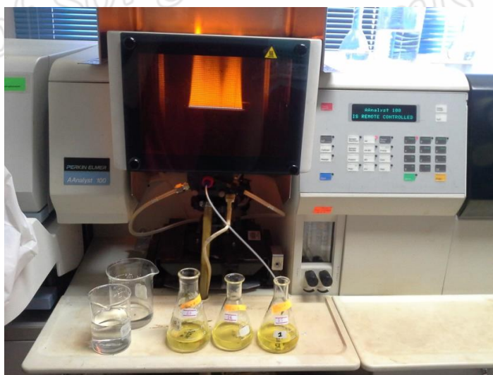
Figure 2. Analysis metal and mineral contents by using ASS 100
