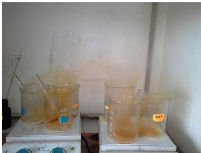
Figure 1. Heating the solution of seaweed and \text{HNO}_3
