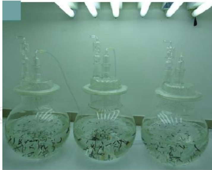
Figure 1.8 G. changii tissue culture in spherical photobioreactor Source: Yeong et al. (2014)
