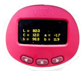
Figure 2: L*a*b measurement by spectrophotometer
