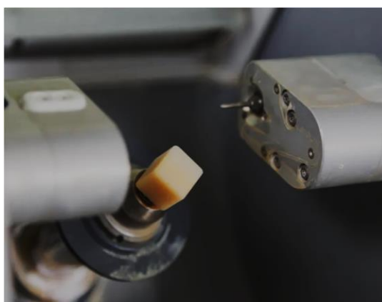
Figure 4: Milling of Vita Bloc® Mark II by CEREC Primemill®
