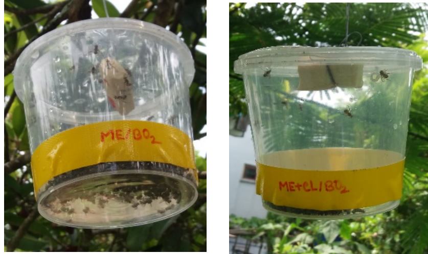
Figure 18. The plastic container trap and trapped flies in the field test
