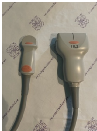
Figure 1.3 The sector/convex/curvilinear 5-8 MHz and linear 3-11 MHz probes
