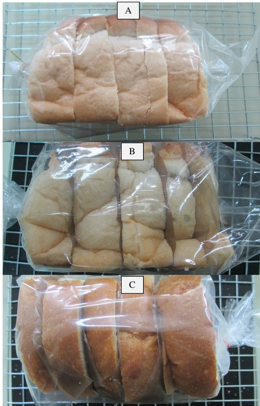
Figure 34 Illustrative of sliced bread treated with various films and packed in PE bags. Without film (A), treated with rice starch films contained OPEFB's lignin (B) and treated with rice starch films contained modified OPEFB's lignin (C).
