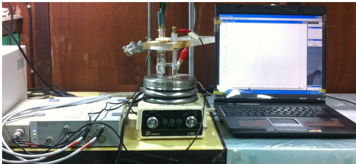
Fig. 2-1 Powerlab 2/20, coupled with Potentiostat (ADInstrument, Australia)
