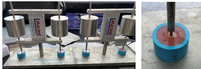
Figure 5. Cementation under a pressure of 750 grams (Gillmore apparatus)
