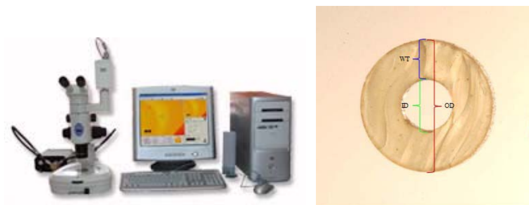
Fig 7. Stereoscopic microscope (Nikon, model smz1500, Japan) and a picture of a ligature during dimensional measurement.
