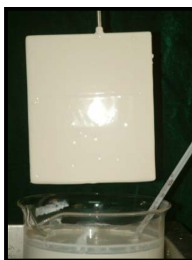
Fig 1. Stainless steel former dipped into heat sensitive compound for rubber thickness of 1.0 mm.
