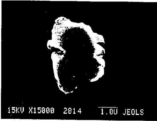
Fig. 7. SEM image of a 3 to 4- \mu\text{m} Yarrabee coal particle after compression.
