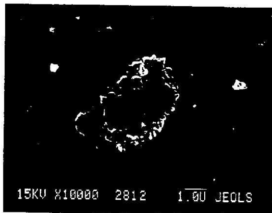
Fig. 6. SEM image of a 1 to 2- \mu\text{m} quartz particle after compression.
