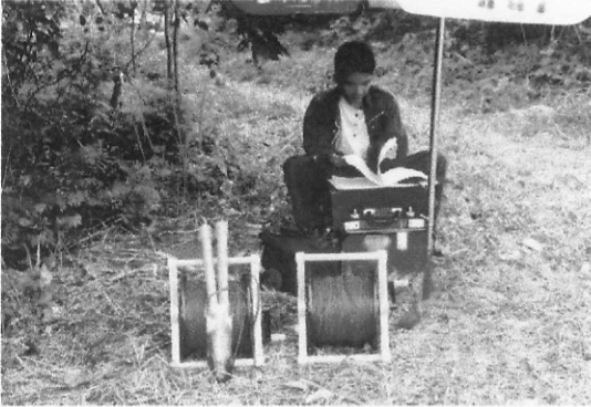
รูปที่ 3.5-2 The SP measurement system consists of two unpolarized electrodes, electrical wires and a terra meter SAS 300 C. One operator at the centre controls the measurements.
