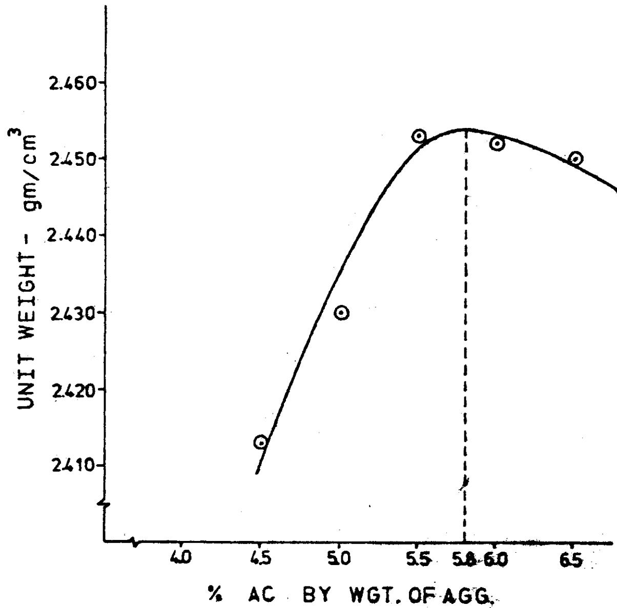
FIGURE 9. VARIATION OF UNIT WEIGHT WITH ASPHALT CONTENT
