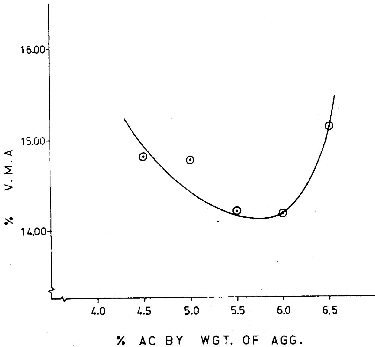
FIGURE 11. VARIATION OF VMA WITH ASPHALT CONTENT
