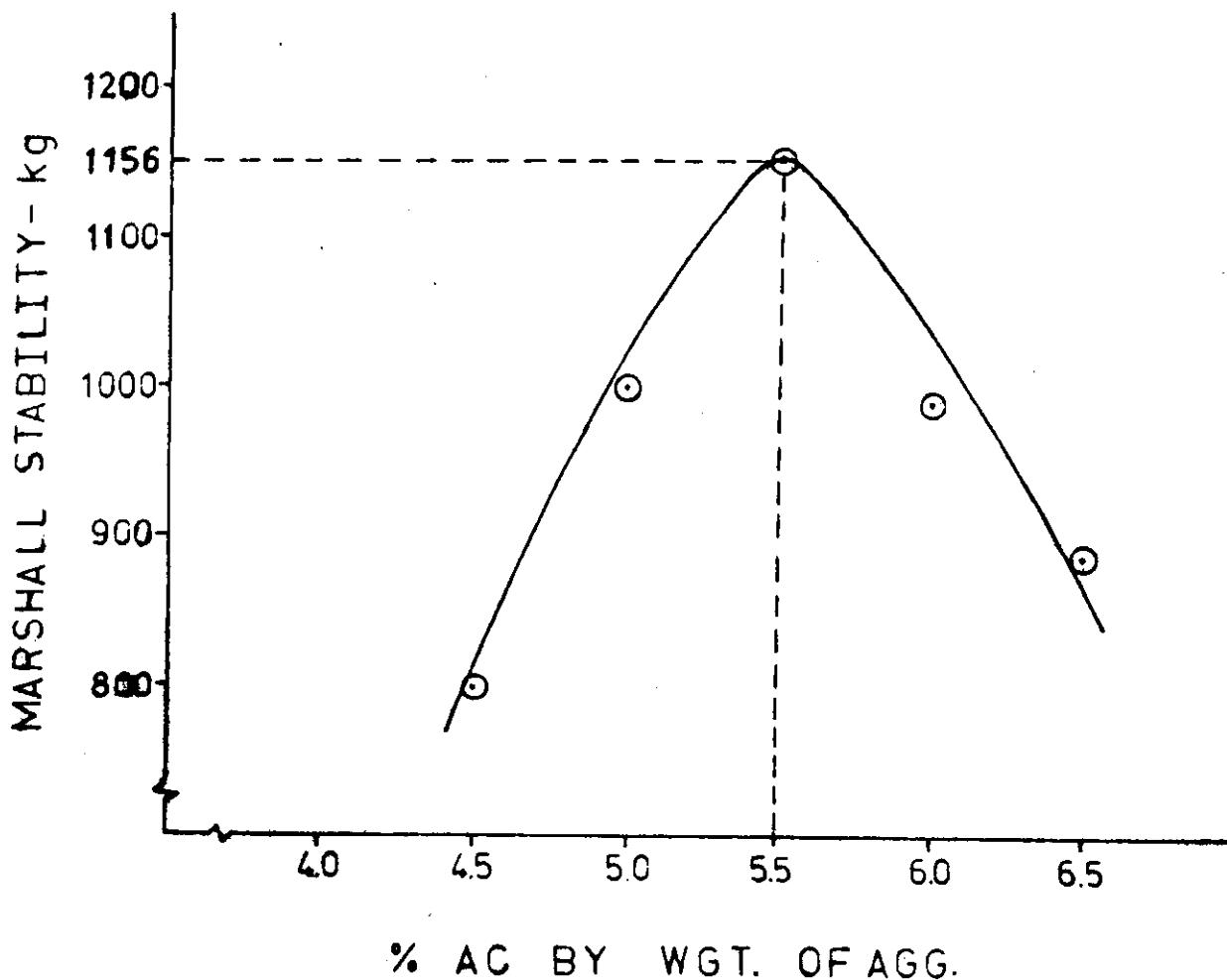
FIGURE 7. VARIATION OF MARSHALL STABILITY WITH ASPHALT CONTENT
