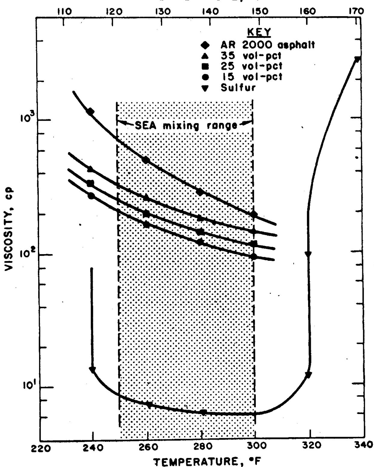
FIGURE 13. SEA MIXING TEMPERATURE RANGE (after McBee 1980)
