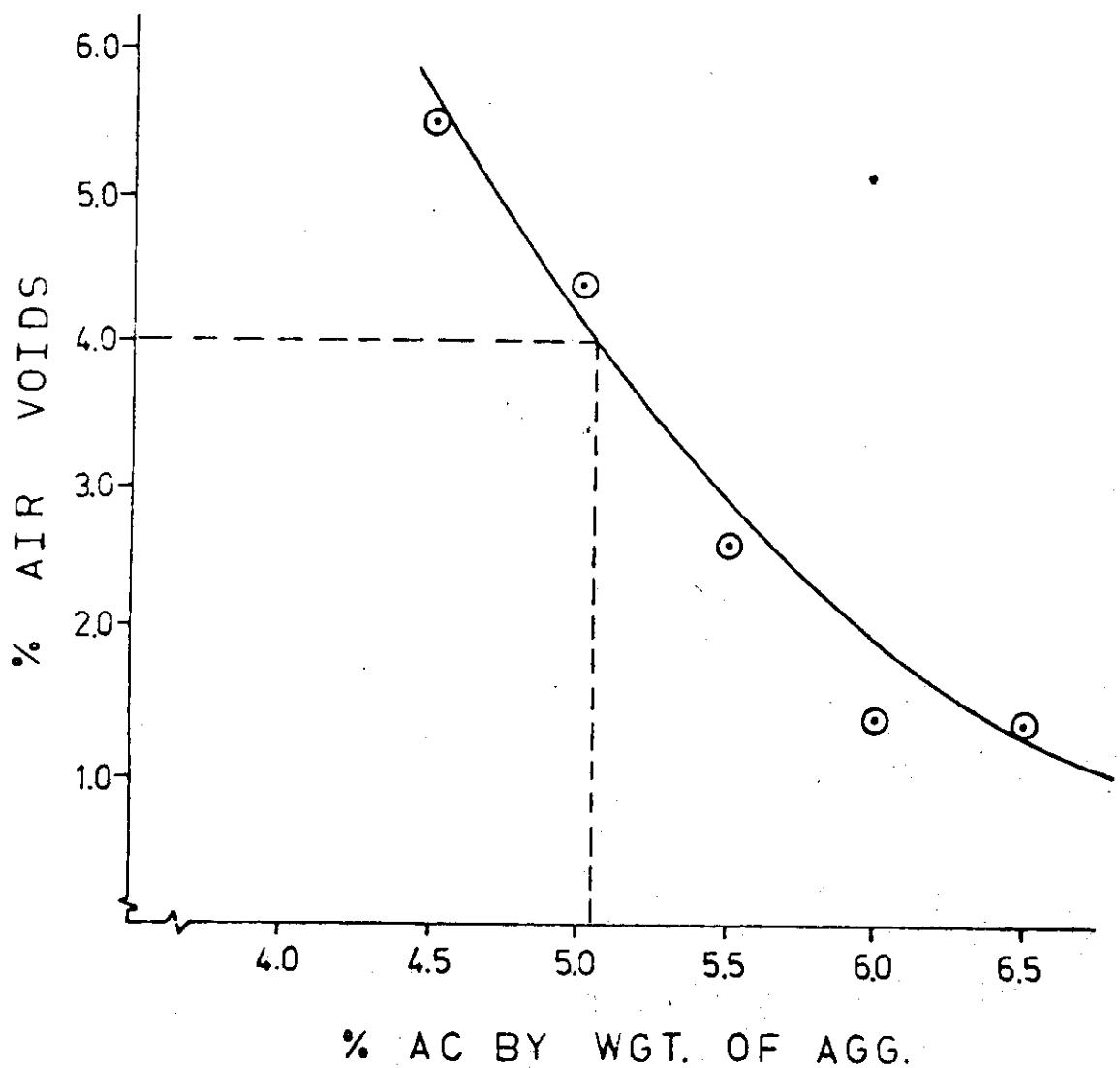
FIGURE 10. VARIATION OF AIR VOIDS WITH ASPHALT CONTENT
