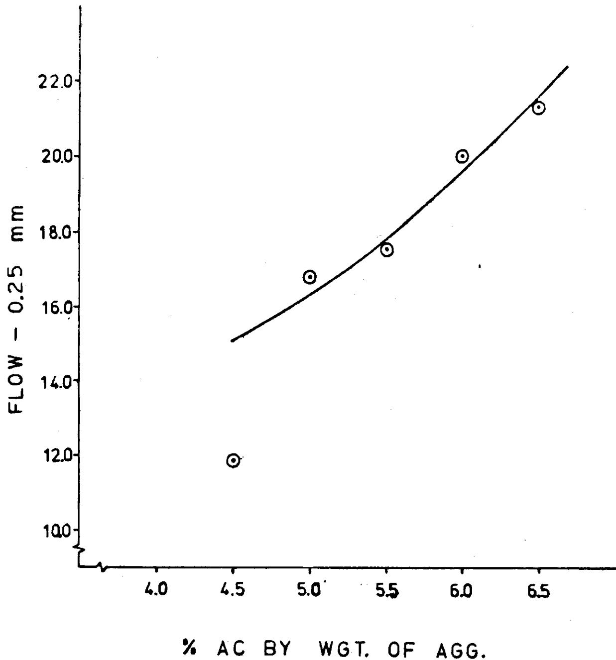
FIGURE 8. VARIATION OF FLOW WITH ASPHALT CONTENT
