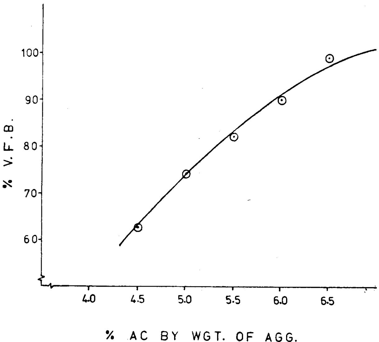
FIGURE 12. VARIATION OF VOIDS FILLED WITH BINDER WITH
