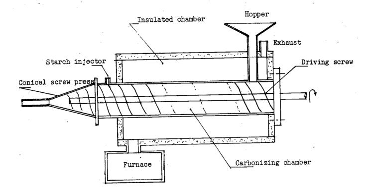
Figure B.1 Conceptual design of leaf carbonization apparatus
