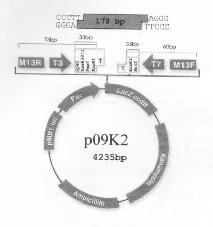
Fig. 2 Restriction map of plasmid P09K2 with synthesized hEGF gene
