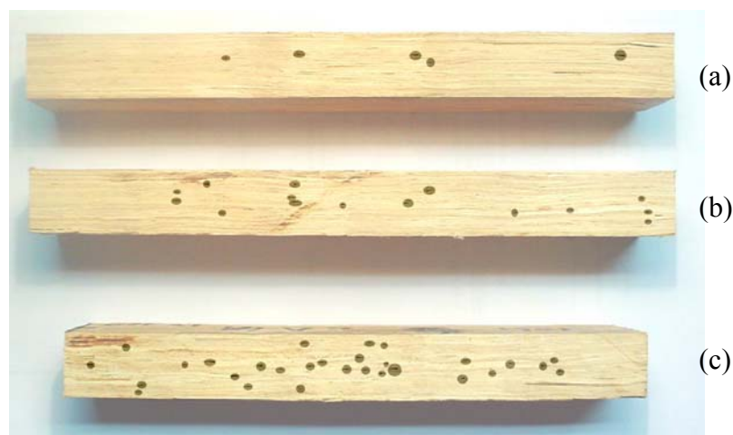
Fig.4.17 Numbers of voids in OSL (shown in black points) comparing between 3 strand length (a) 15 cm (b) 10 cm (c) 5 cm.
