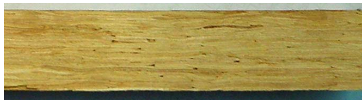
Fig.4.16 Voids in OSL manufactured in laboratory
