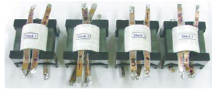
Fig. 5 Experimental high frequency transformers
